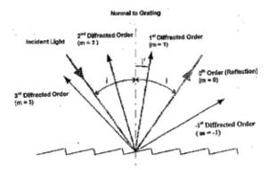
A diffraction grating is an optical component with a regular pattern of elements or grooves. All gratings have intensity maxima at angles  $\theta_m$  which are given by the grating equation
