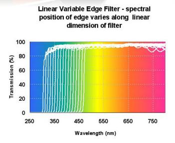
Barr designs and manufactures both edge-type and bandpass-type LVF's to customer specifications, and both types of LVF's are sometimes used as Order Sorting Filters in grating-based systems. For example, a Linear Variable Filter can be used in an imaging spectrograph to provide order sorting when used with a focal plane detector.
