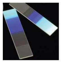
A Linear Variable Filter (LVF) is comprised of an interference filter coating on a glass or fused silica substrate deposited in such a way that the spectral properties of the filter vary continuously and linearly along one of the linear dimensions of the filter.
